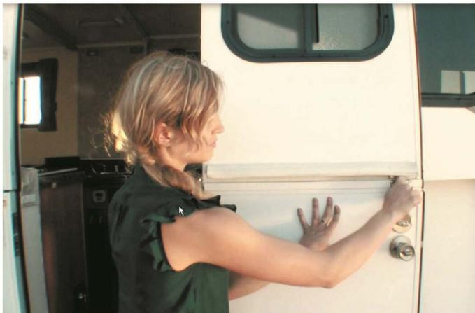
**Step 11:** Open bottom door section fully and latch to top door section. (door sections usually fit best when in fully opened position). Slide entrance step out and lower second step, then enter unit.
