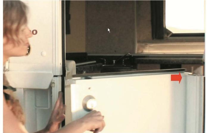
**Step 10:** Open bottom door section, and push outward until pin in the right door frame latches to trailer.
