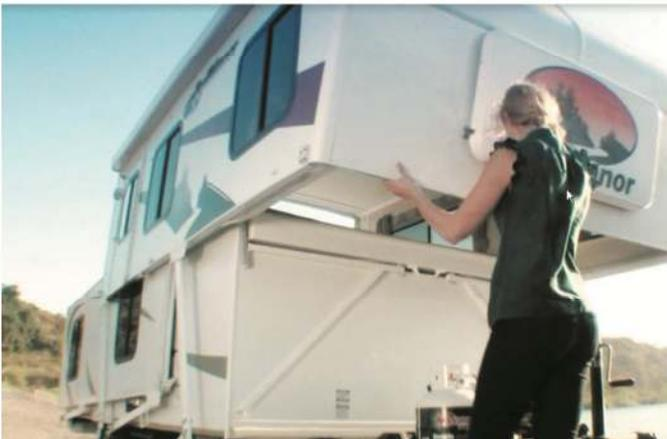
**Step 3:** Standing near the tongue, grasp the lower edge of the front roof section. Lift the front roof up and out in a circular motion beginning with a straight-up motion and finishing with a pull. **Do not lift the roof by the front window stoneguard. Do not lift by the sides (risk of pinched fingers).**
