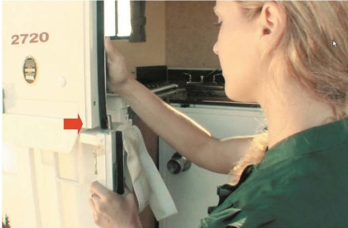
**Step 9:** Push the left bottom door frame out and latch against pin. Fold Velcro flap over inside trailer.
