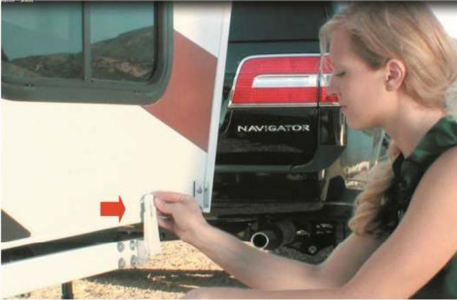
**Step 1:** Release the four white draw latches, one at each corner of the trailer.
