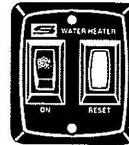
The thermostat-limit controls the power to the module board. At a preset temperature the thermostat will open shutting off the burner. If the thermostat fails, the limit or ECO switch will open and must be manually reset.
