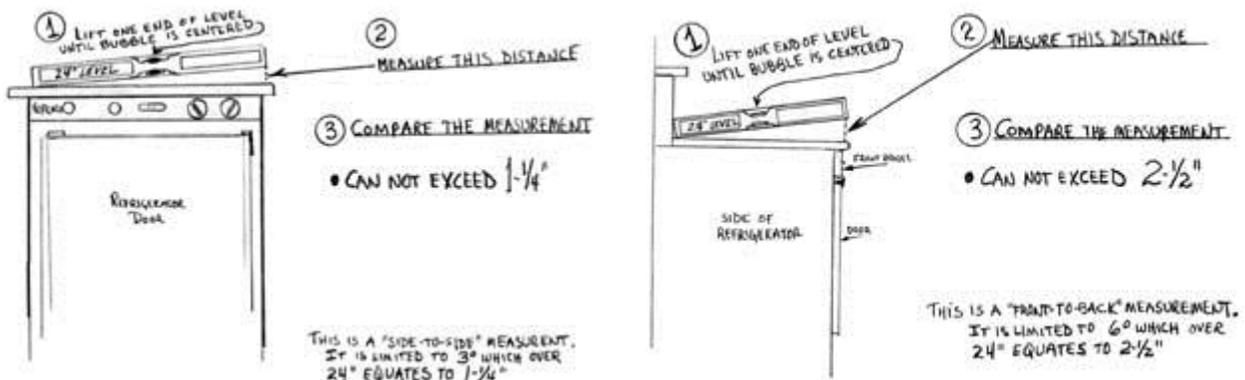
It is apparent that the refrigerator is supposed to work properly even when it is well beyond what we all thought were the limits for out-of-level condition. And after viewing those sketches, you are probably asking yourself "Why bother leveling at all?" Well, Norcold states the answer simply as *"Normal vehicle leveling to provide comfort for the occupants is satisfactory for refrigerator operation"*.
