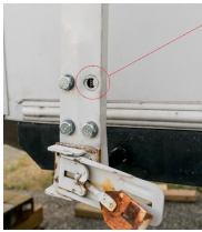
Partial collapse of pocket. Note bulge.
