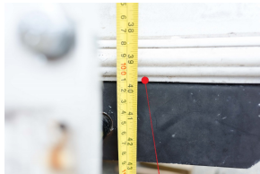
Measure to bottom of trailer (39.5"). (I set mine to 39.75" to compensate for partial pocket collapse, discussed later.)
