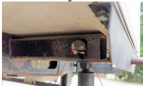
Worm clamp in place Missing washer
