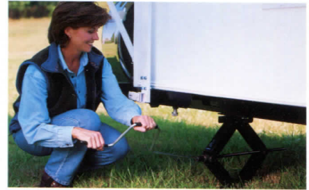
Standard Scissor Jacks Four standard scissor jacks make leveling simple and fast.
