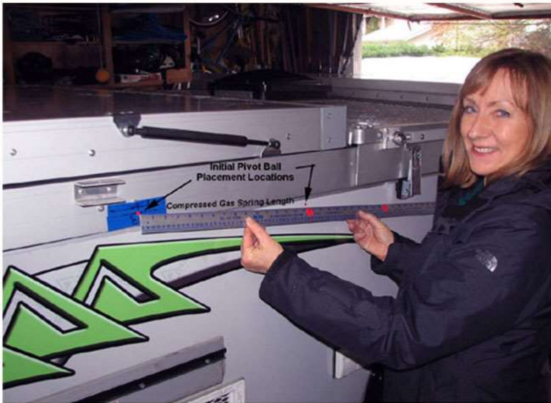
Initial Pivot Ball Placement Locations (Roof Panels Lowered)
