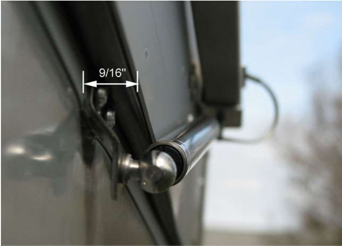
Maximum Edge Spacing for Shim-free Installation
