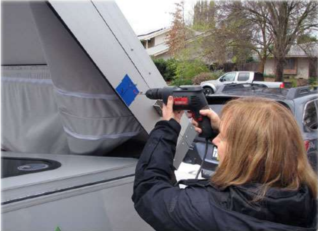
Drilling the 5/16" Diameter Upper Holes for the 10 mm Ball Studs
