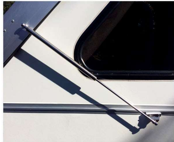
New Gas Spring Installed!
