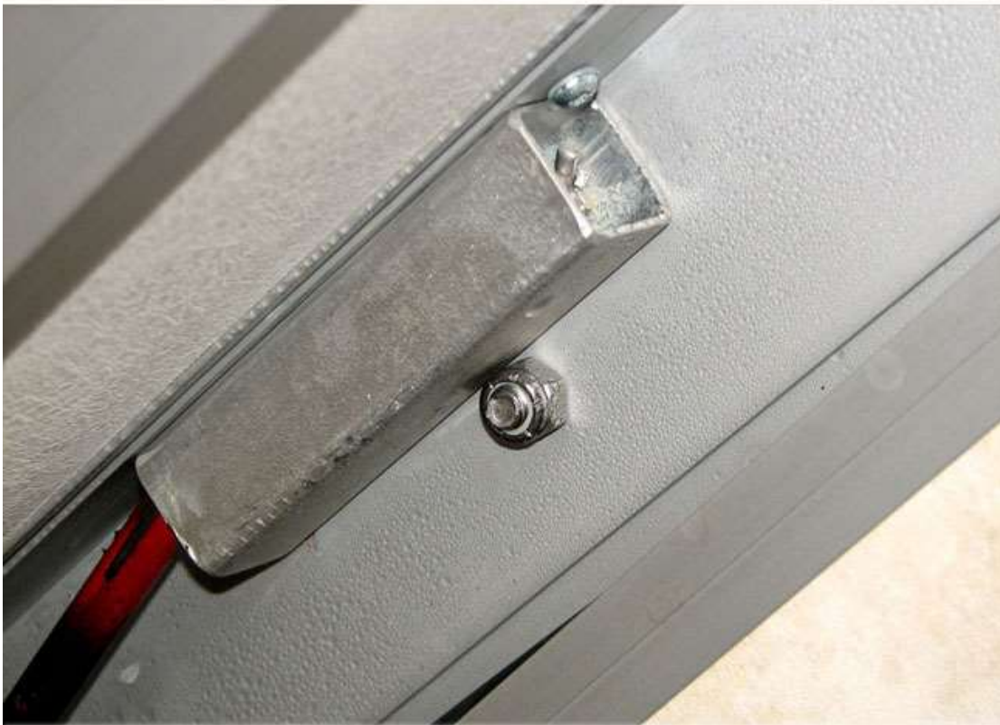
Nylock Nut on 5/16" x 18 TPI Stainless Steel Threads for Ball Stud
