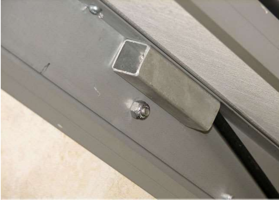
Nylock Nut on 5/16" x 18 TPI Stainless Steel Threads for Ball Stud
