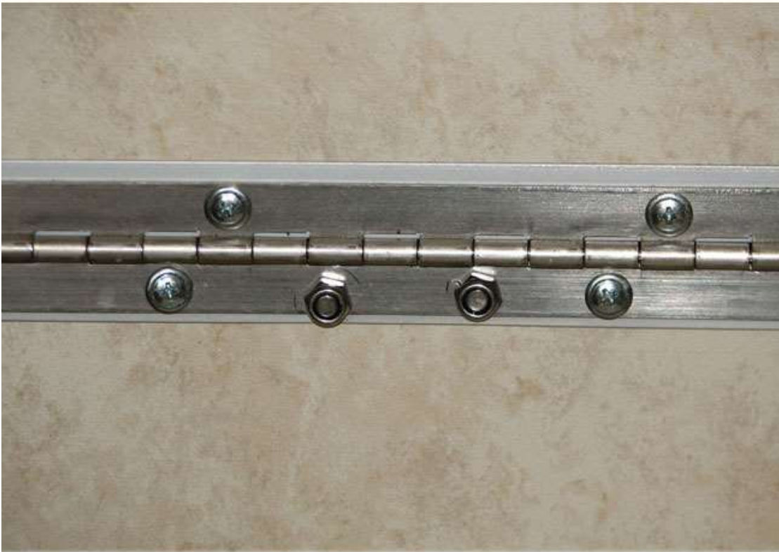
Nylock Nuts on 40 mm Stainless Steel bolts for Offset Brackets
