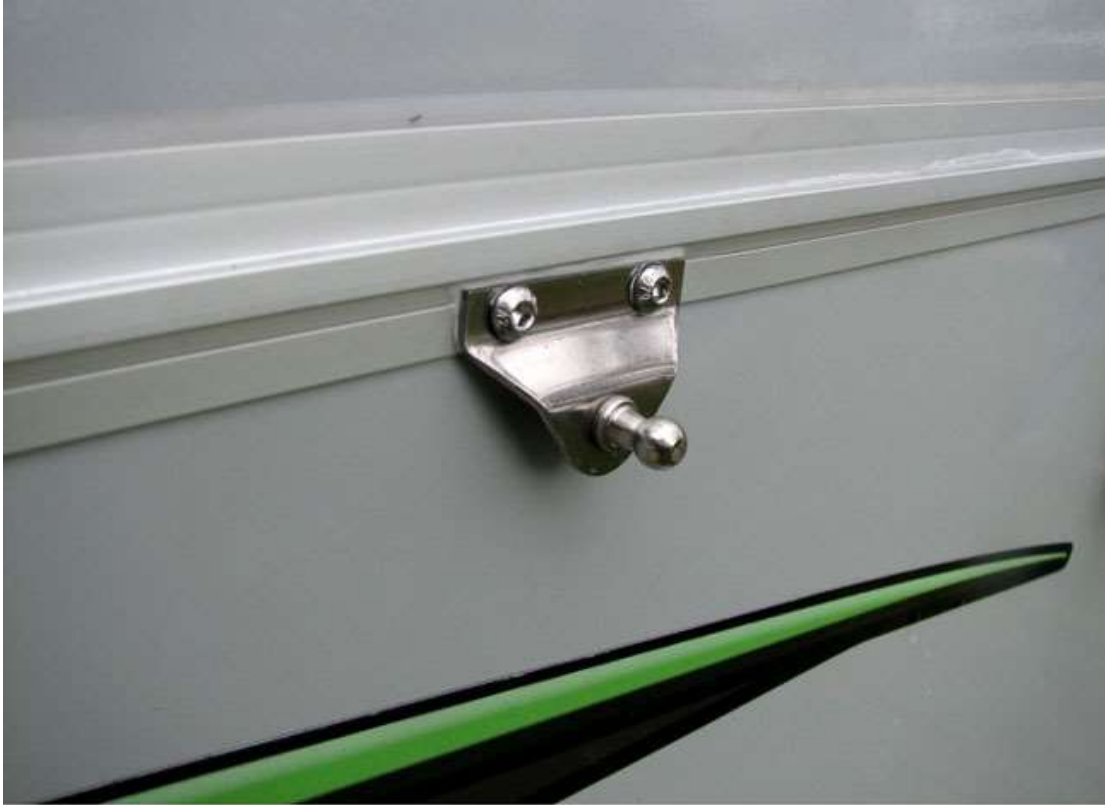
New 10 mm Stainless Steel Offset Bracket (no Shim Required)
