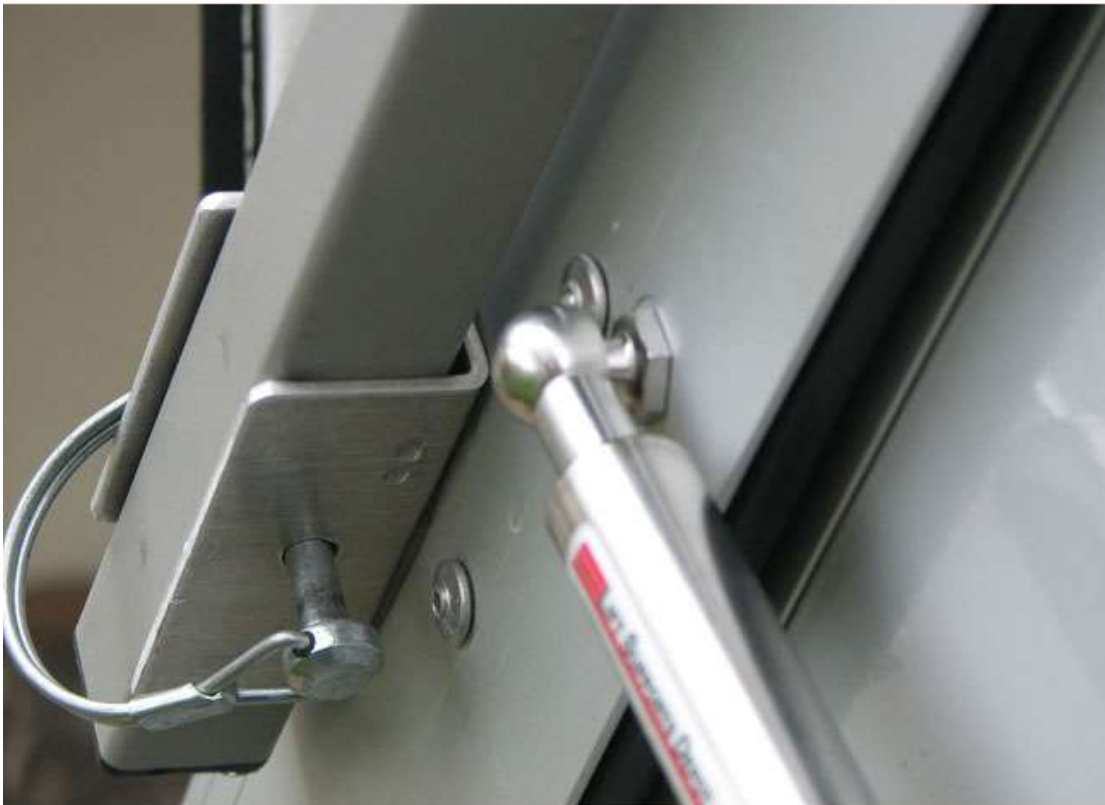
New 10 mm Stainless Steel Ball Stud & 30 Pound Gas Spring
