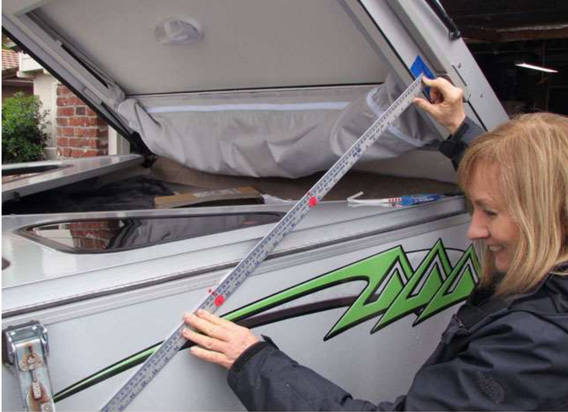
Checking for Proper Pivot Ball Placement (Roof Panels Raised)
