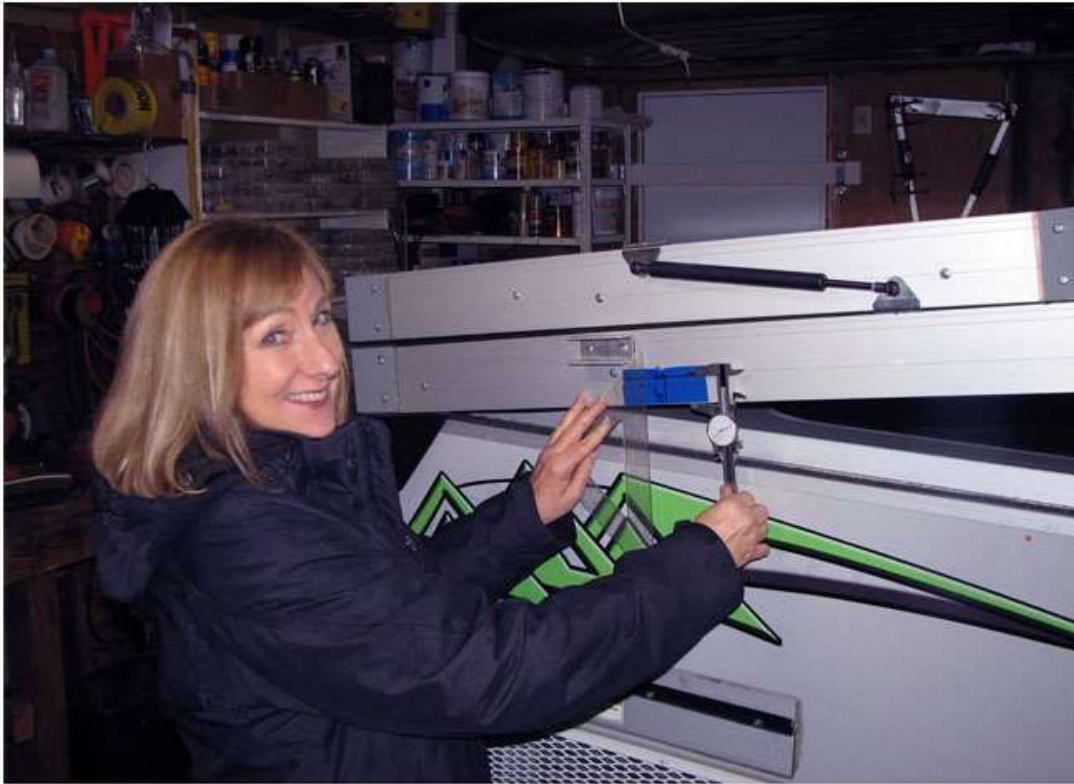
Marking Upper Obstruction Line & Starting Line (19" from Hinge)
