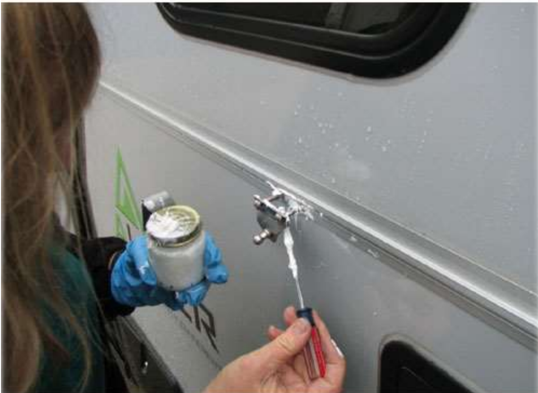
Applying 3M Adhesive Sealant for Waterproofing
