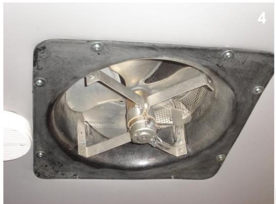
Use a jig saw with a medium course blade and cut with the slowest strokes possible. If you cut at high speed, the plastic welds itself back together. The entire weight of the vent is on the screws that hold the base to the ceiling. Use large washers under the screws to distribute the stress of the wind on the vent at highway speeds.
