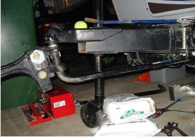
Trailer Hitch with truck down driveway with equalizer hitch adjustment plate setting at 5.
