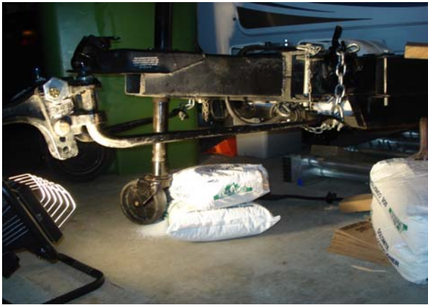
Hitch plate adjusted to maximum setting of 6 to give 2 more inches of clearance of round bar to swing hitch plate.
