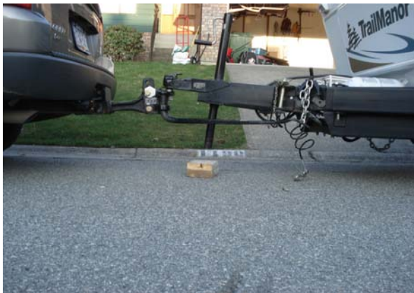
Adjusted hitchbar set 2 inches higher 19 inches to match level setting of trailer at 19 inches from ground
